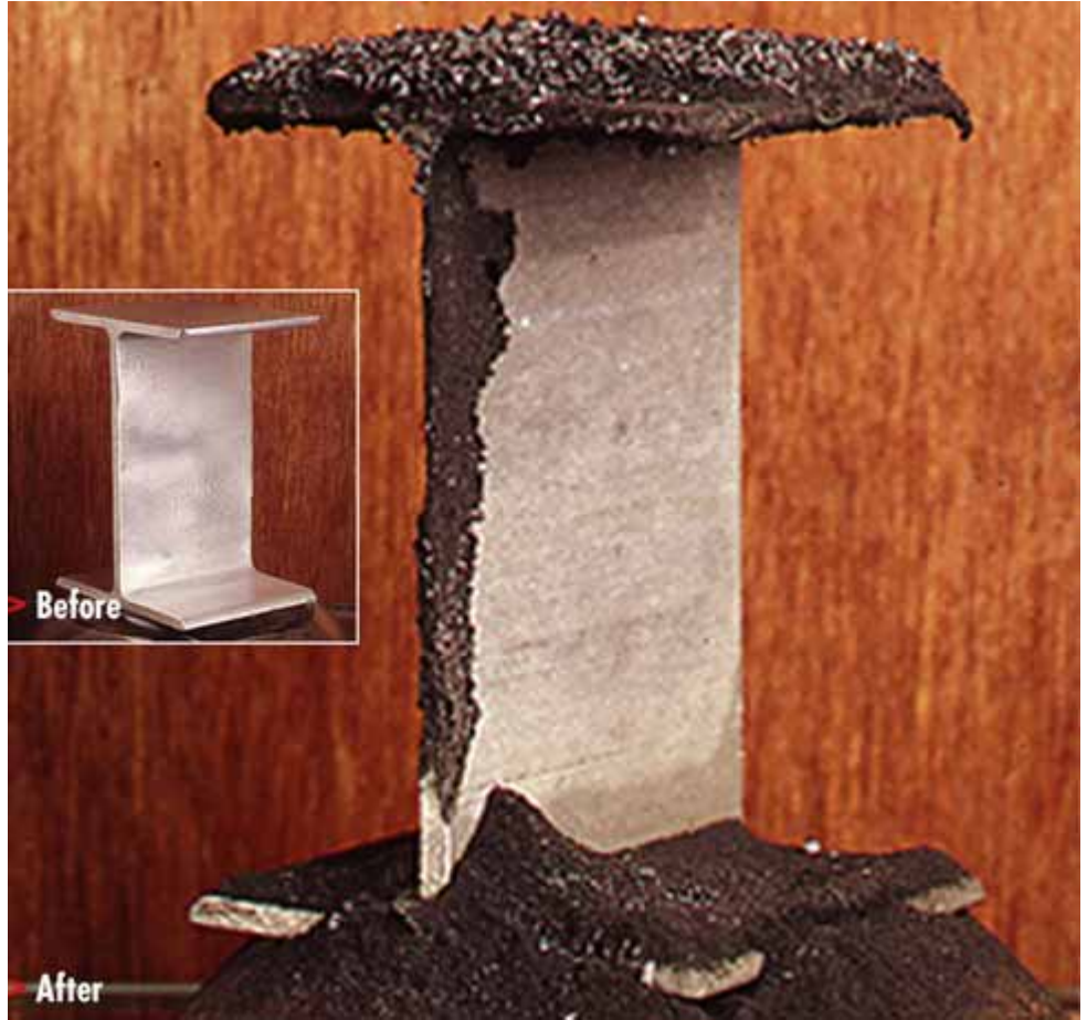
Just a small amount of mercury paste starts turning this aluminum I-beam to dust.
