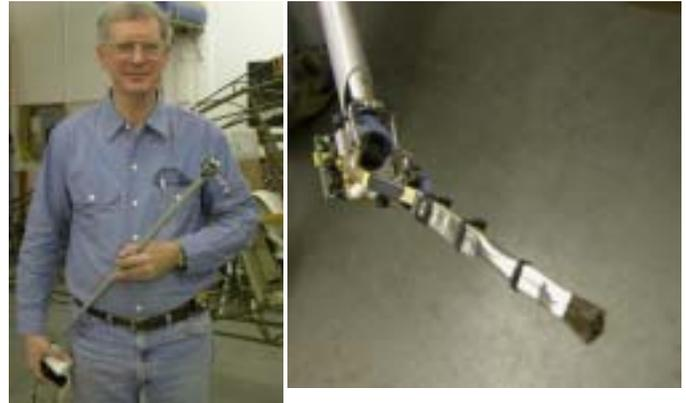
The business end of the "Remote Dauber" consists of a brush which can be rotated and swept back and forth by a handle on the other end of the concentric tubes while watching on a TV set. The TV camera is on the bottom in the detail photo. Scott says that the sealing compound is thick and difficult to apply.
