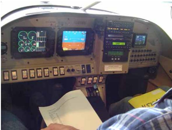
Notice the Dynon backup display on the right panel. This is the same type of display that was used in Space Ship One for the successful at-
